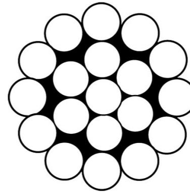
BOBINE CABLE MONOTORON
